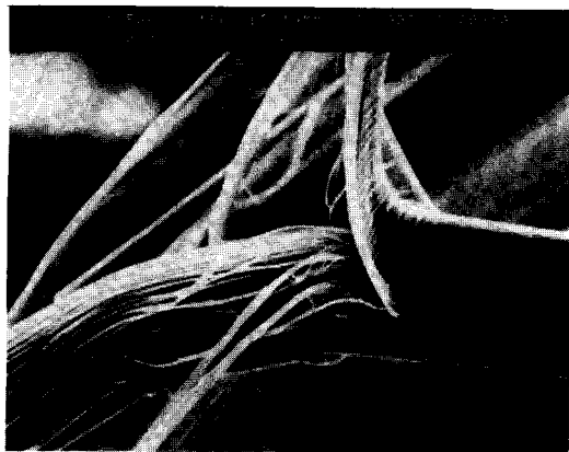
Figure 8 SEM micrograph of single fibre tested in transverse testing device
