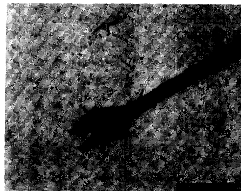
Figure 5 Optical micrograph of single fibre which has been flattened and then had a notch created in it using a micromanipulator
